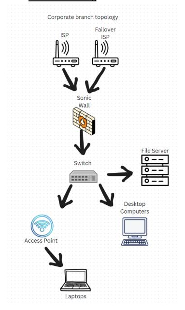
Each device on the corporate network currently sends traffic from their device through the switches, through the firewall, then out to the internet. Any inbound and outbound traffic is monitored, but the monitoring leaves a lot to be desired since the current firewall is out of date.
