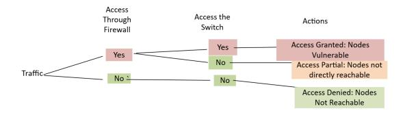
This decision table shows the traffic's ability to gain access to nodes within the network. If the traffic can make access through the firewall, then the traffic meets another decision. It will need to access the switch to directly access the nodes. If the traffic cannot make access through the firewall, then it will be unable to access the switch. Today, the traffic can access through the firewall and the switch.
