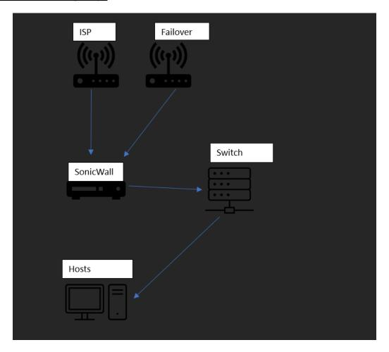
Currently the point-of-sale equipment piggy backs off the desktop computer's internet connection and sends all transaction data over a peer-to-peer encrypted tunnel to the transaction company. All other devices send their data through the network, out the firewall, and out to the internet. The issue with the current firewall is that it is out of date and needs to be upgraded to a
