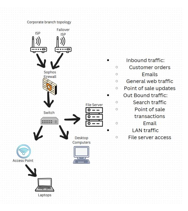
Each device on the corporate network currently sends traffic from the device through the switches, through the firewall, then out to the internet. All inbound and outbound traffic is monitored, but the monitoring leaves a lot to be desired since the current firewall is out of date.
