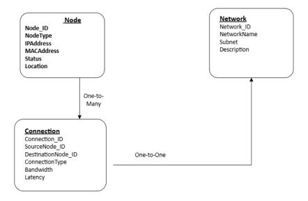
The node would be the main entity in this diagram. The node creates connections to communicate. Those connections are communicated through a particular network. The node can have various connections at one time, but the connections can only be on one network at a time.
